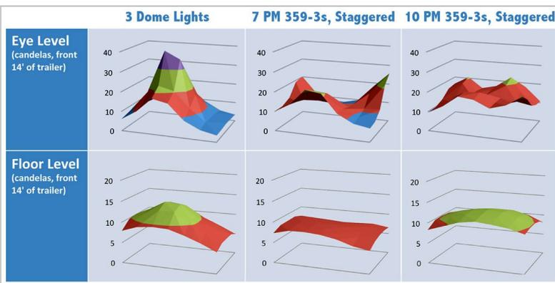
Photometric data proves that the new 359 interior lighting system provides more efficient, more evenly distributed light through the vehicle compare to recessed ceiling units.
